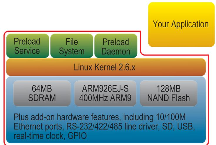
With pre-installed Linux OS, users can easily operate Matrix-518 via Telnet, or transfer files using FTP.
